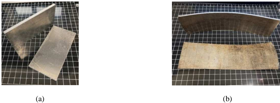
Figure 1 : (a) As-received 5083 Al alloy and (b) Ultrafine-grained 5083 Al alloy
