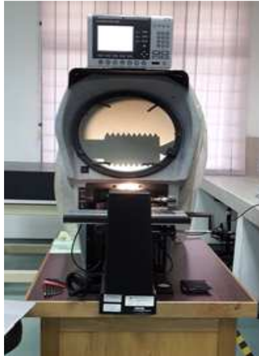
Figure 5: The 14' Horizontal Beam Comparator.
